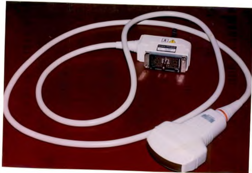
Aloka SSD-500 ultrasound scanner and 5.0MHz curvilinear transducer mainly used in this study
