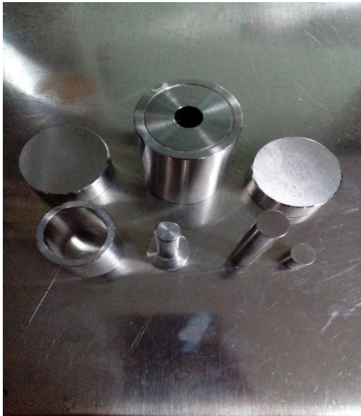
Figure 3.4 Die and its parts.
