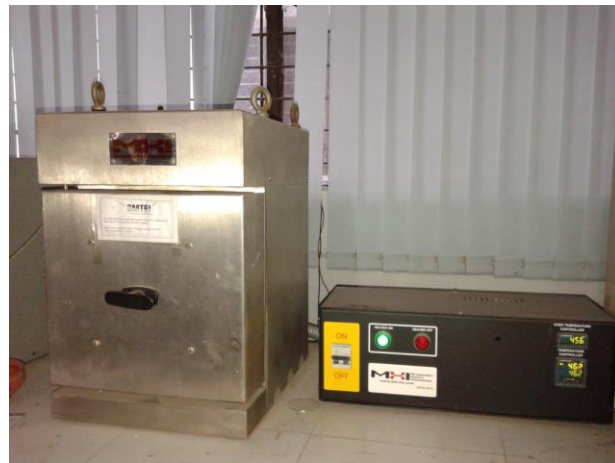
Figure 3.8 A high temperature furnace (MHI Corp., BPAN-2010, USA).
