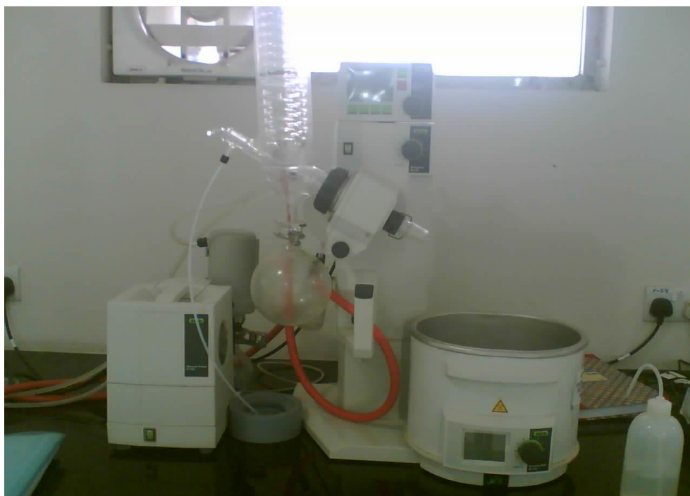
Fig 2.2: Rotary vacuum evaporator
