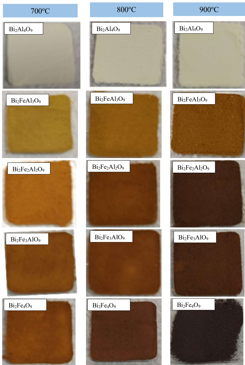
Fig. A.2.5. Optical appearances of \text{Bi}_2\text{M}'_y\text{M}''_{4-y}\text{O}_9 at different temperatures and compositions.
