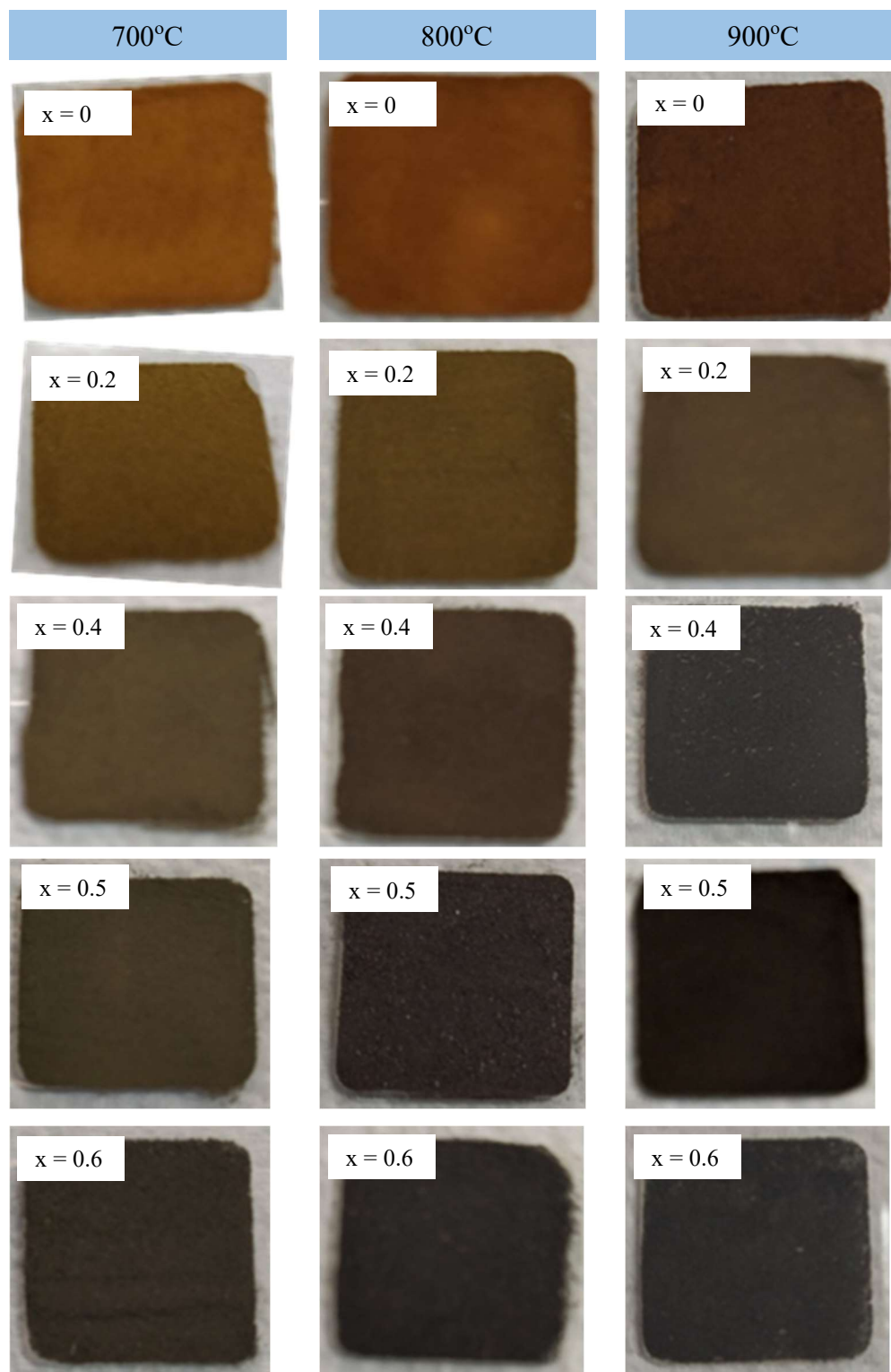
Fig. A.2.8. Photographs of \text{Bi}_2\text{Fe}_3(\text{Cr}_x\text{Al}_{1-x})\text{O}_9 prepared at different temperatures.
