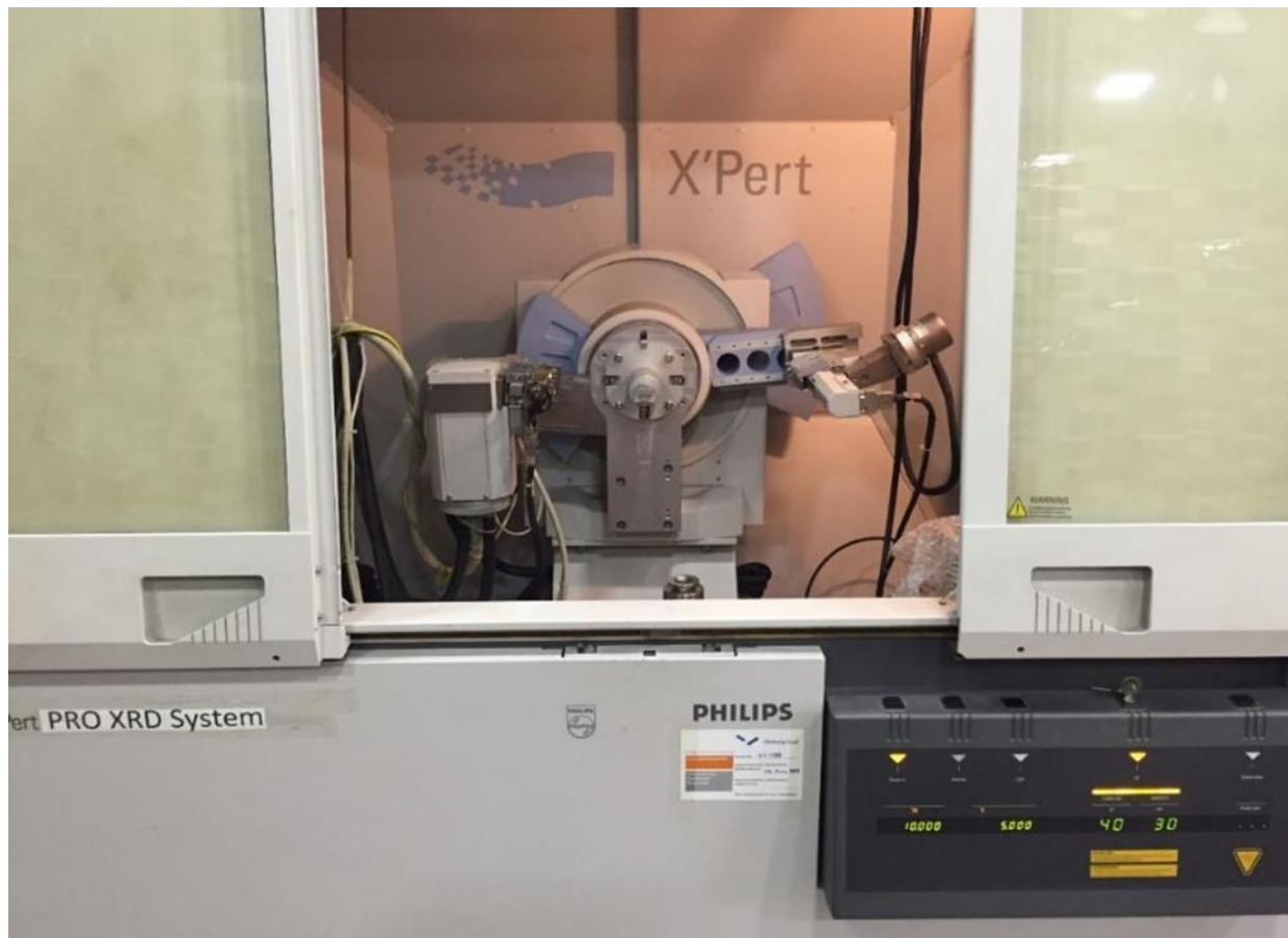
Figure 3.4: Philips X'pert PRO X-Ray Diffractometer (PW3040) at materials science division of Bangladesh Atomic Energy Commission.
