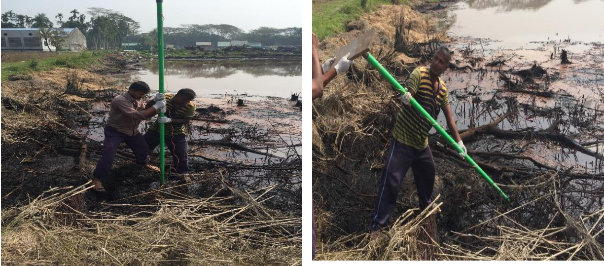
Figure 5.4: Sediment sample collection process from the WDEvp Pond of GF by using acrylic pipe.
