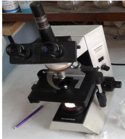
Figure 6. Compound microscope (Olympus, Model-CH30RF200, Japan) is for viewing zooplankton
