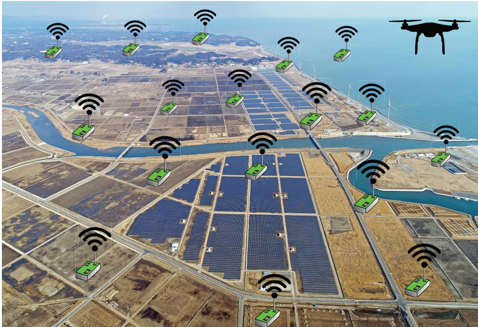
Figure 1.6: A sensor network to monitor solar panels with a mobile sink [3]
