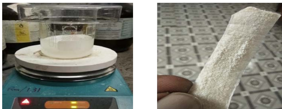
Fig.2.7. Preparation of sulfonated adsorbent from non-woven polyethylene film.
