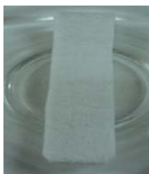
Fig. 2.9. Sulfonated-GMA-PE film before adsorption
