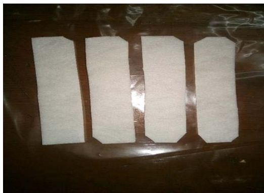
Fig. 2.5: Non-woven polyethylene film (8 cm×1.5 cm).
