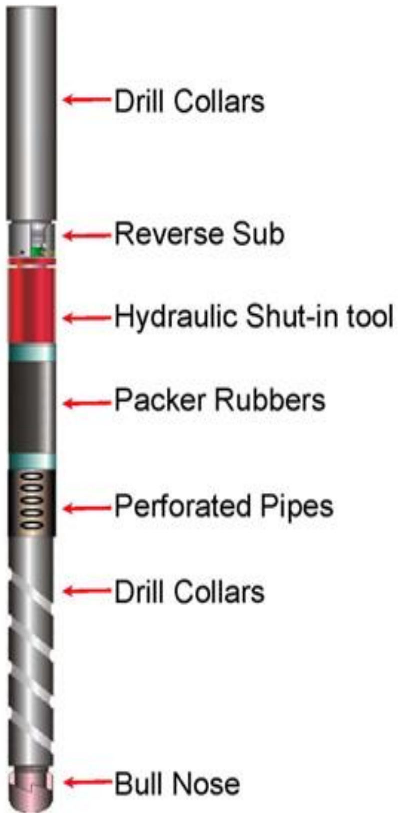
Figure 4.8: DST string and BHA for DST operation.
