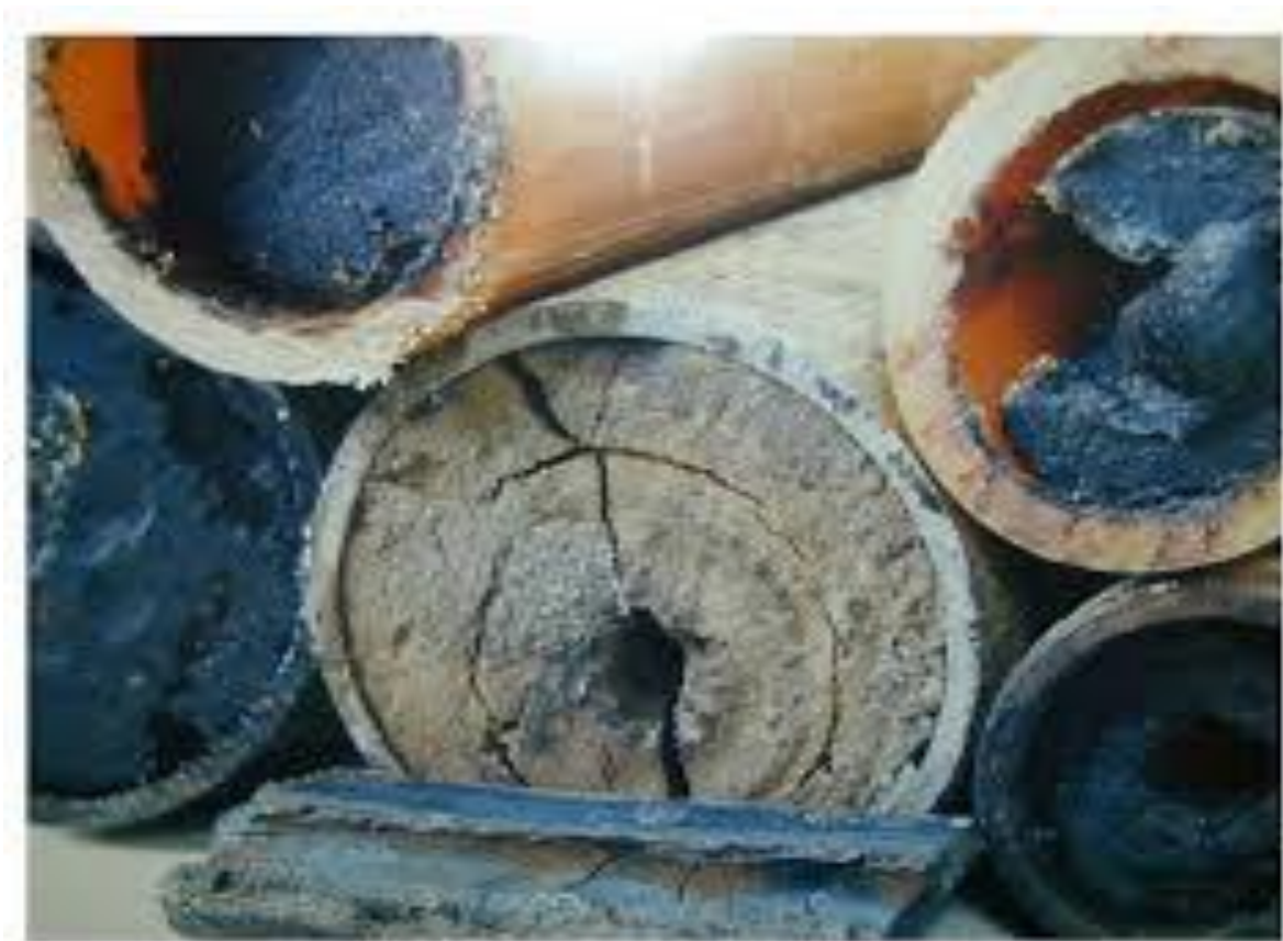
Figure 3.68: Scale and wax deposition in production tube
