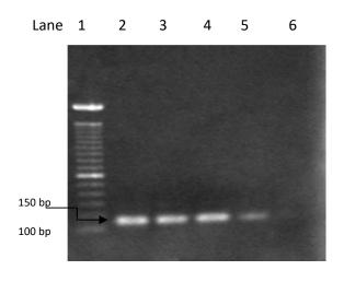
**Fig. 8.** Agarose gel electrophoresis showing 150 bp amplification products of *eaeA* gene specific primers. Lane 1-100 bp marker, lane 2- positive control, lanes 3 to 5- Isolates, lane 6-no template (negative) control.
