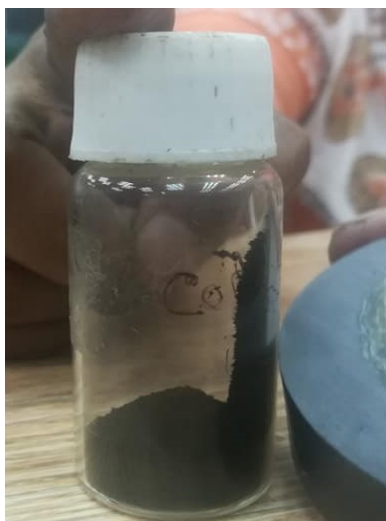
Figure 3.2: Synthesized cobalt ferrite nanoparticle's attraction to magnet
