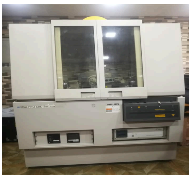
Figure 3.8: Philips X'pert pro XRD (PW3040) at materials science division in Bangladesh Atomic Energy Commission.
