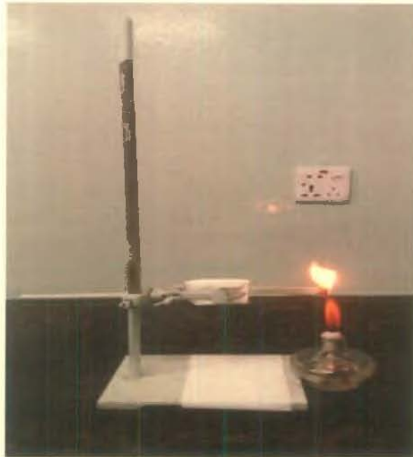
Figure 8.1: Ignition time and total firing time experiment.
