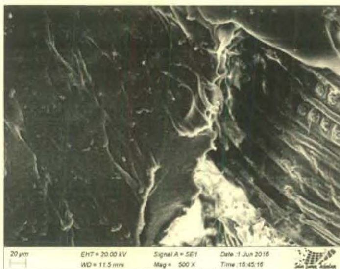
Figure 7.14: Image of (90% PP + 10% ALS) fibers reinforced polypropylene composites.
