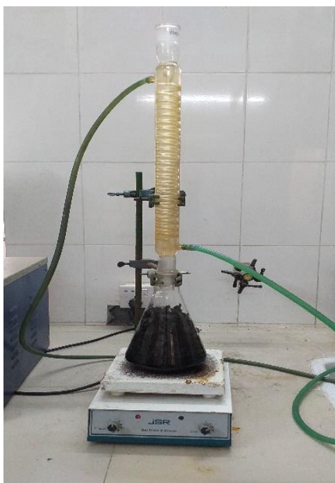
Figure 4.2. Experimental setup for formic acid cooking
