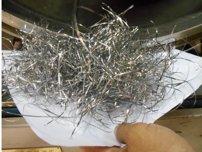
Figure 4.1:(b) Prepared ribbons by melt spinning system.
