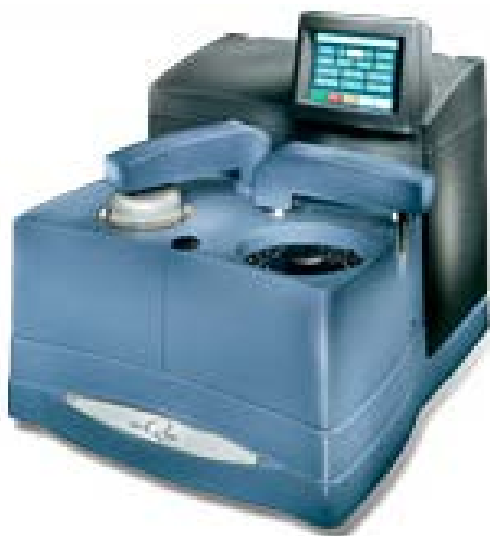
Figure 4.2: Set up of differential scanning calorimeter.
