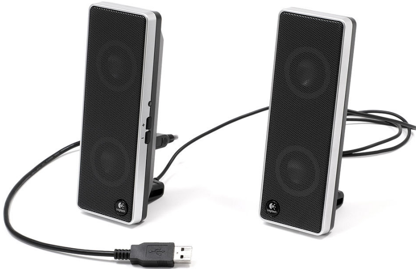
Figure 7: A pair of speakers for notebook computers that are powered and audio-connected to the computer via USB. Source: https://en.wikipedia.org/wiki/Computer_speakers
