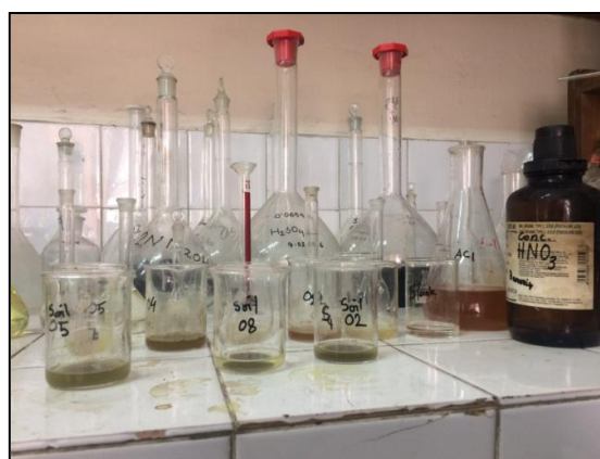
Illustration 6.11: Preparing the Grinded Mollusk Shell Samples for digestion
