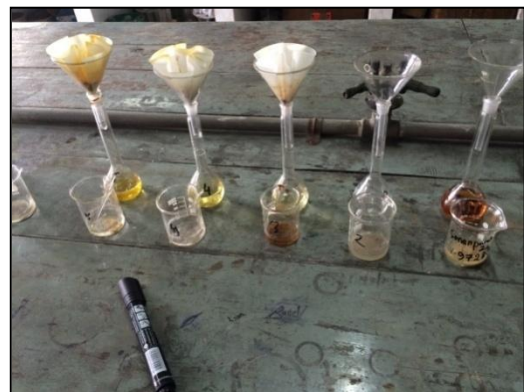
Illustration 6.4: Filtering the Digested Soil Samples
