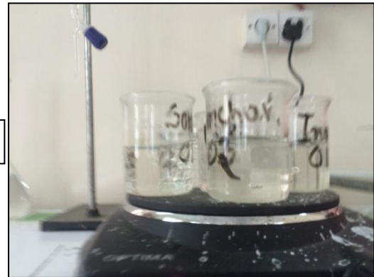
Illustration 6.2: Digestion of Water Samples
