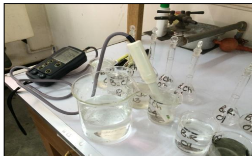
Illustration 6.7: Measuring the Physio-Chemical Parameters of the Samples with Ph Meter
