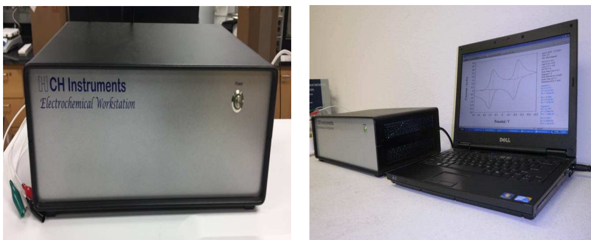
Fig. 2.6: Computer controlled potentiostat used in electrochemical analysis
