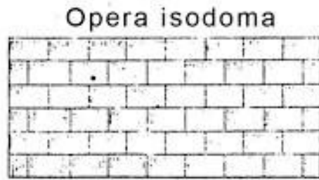
Figure no.- C03. Opus isodomum (left) and opus pseudoisodomum (right)
