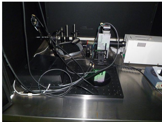
Figure 3.7 Inside View of Spectral Response Measurement System
