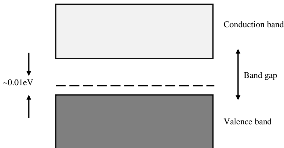
Figure 2.3 N -type Semiconductor
