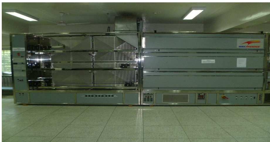
Figure 10.4 POCl_3 Diffusion Furnace
