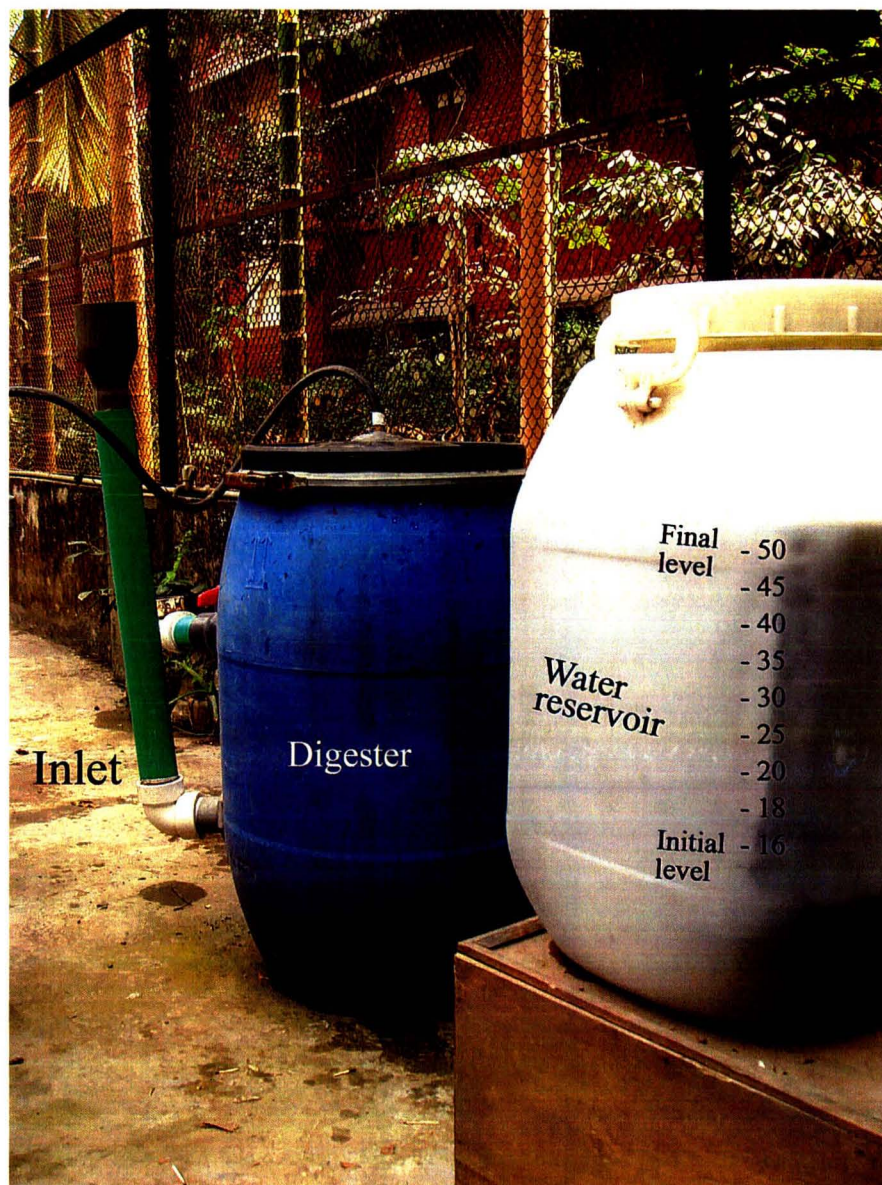
Fig. 2.5. Front view (partially) of the “Mini-Biogas Plant”. The raise of the water level in the translucent plastic reservoir from 16 L up to 52 L mark indicates 36 L of biogas stored in the digester. The 16 L level corresponds to the upper level of substrates in the digester without any gas.
