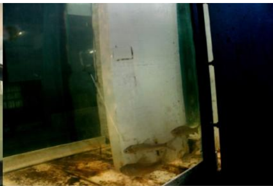
Fig 87. Fishes entering into pass from downstream
