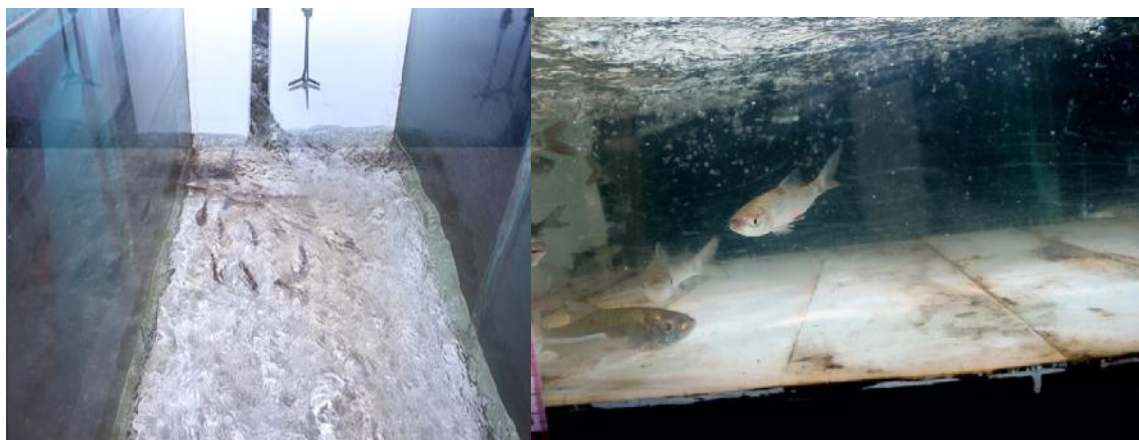
Fig 68. Fishes swimming with the water flow Fig 69. Fish sustained speed in second chamber
