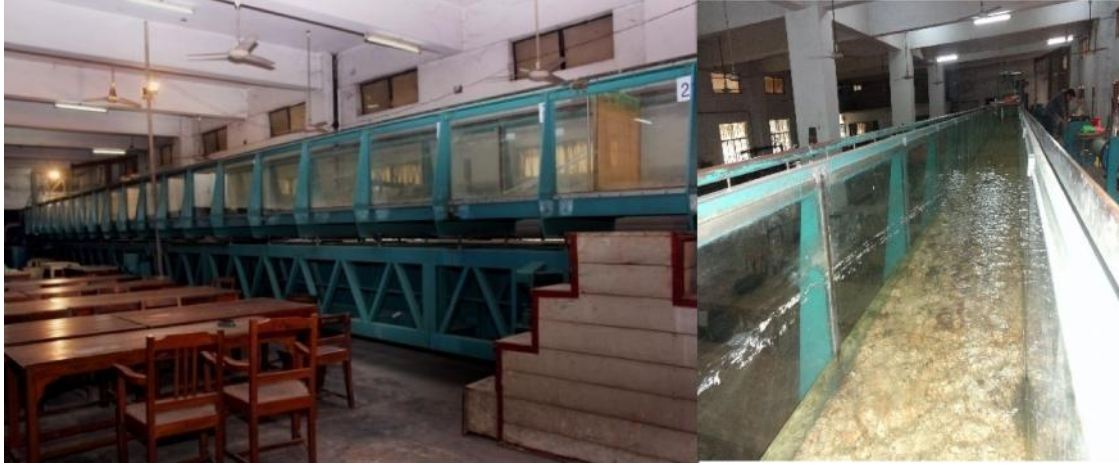
Fig17. Flume used for fish migration study in laboratory Fig18. Inside view of flume
