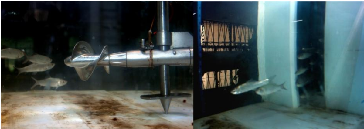
Fig101. Fishes moving around ADV Fig102. Fishes passing from pool 1 to pool 2
