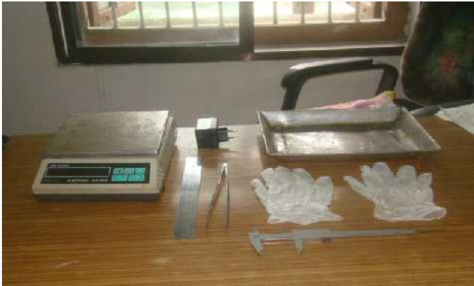
Plate 22. Gloves, scale, slide calipers, forceps and a tray used for measuring
