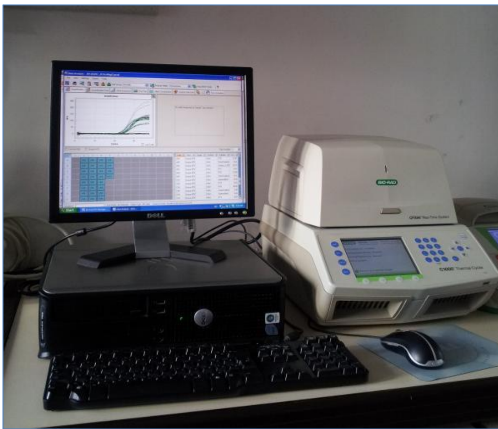
Figure 5.2: BioRad CFX-96 real time system (BioRad, USA) used in the present study.
