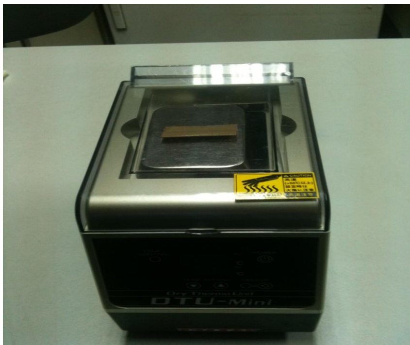
Figure: 6.2: Heat block (heating chamber) used for LAMP assay.
