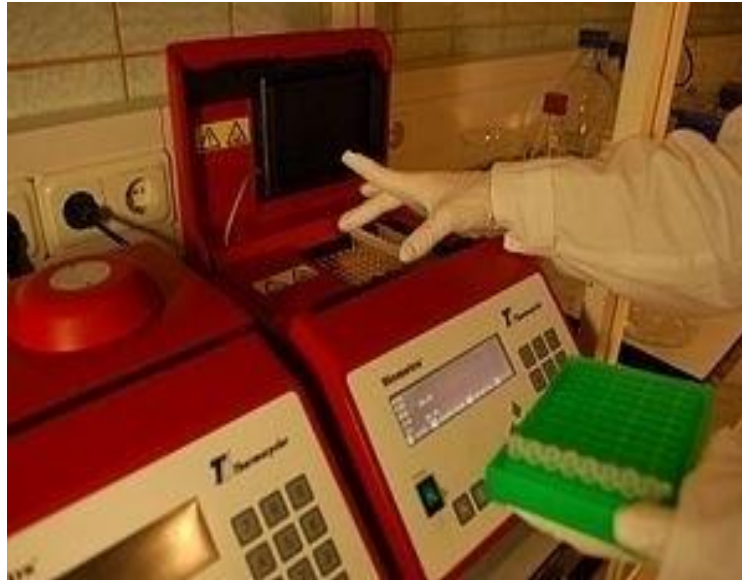
Fig 3.9: Placing a strip of eight PCR tubes, into the PCR machine
