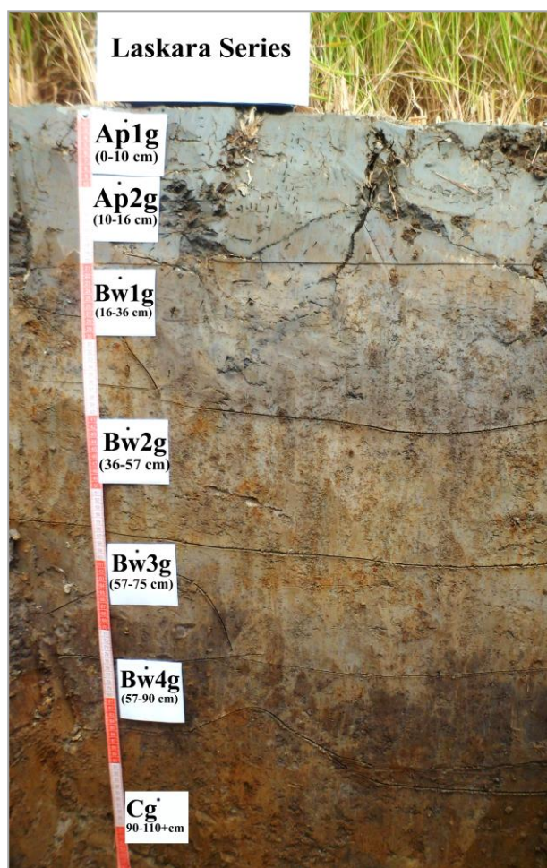
Plate 15. Profile of the Laskara soil series formed on the lower Atrai basin.
