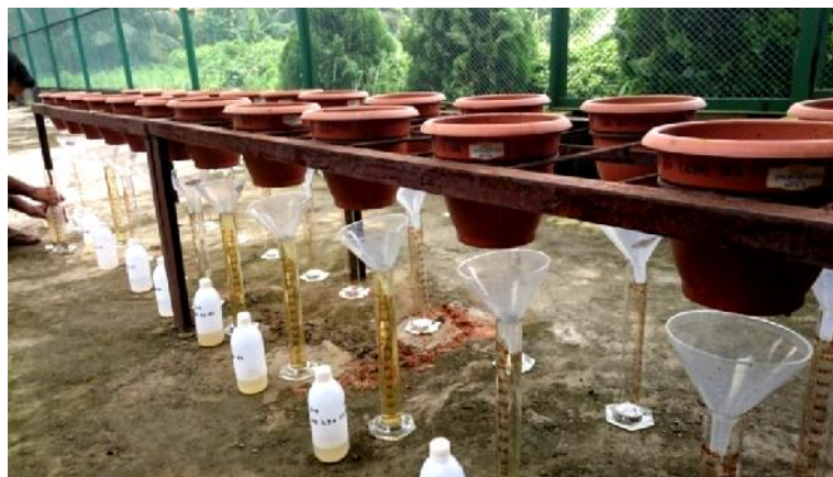
Fig 3.11. Collection of leachate after extraction with fulvic acid and combined extractant
