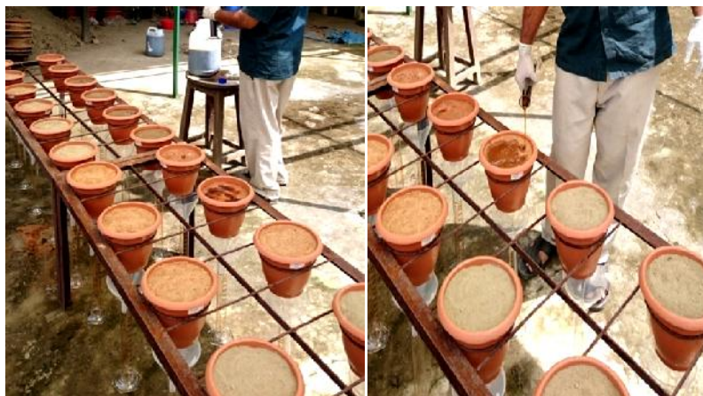
Fig. 3.9. Application of humic acid, fulvic acid and mixed suitable extractants to contaminated soil.
