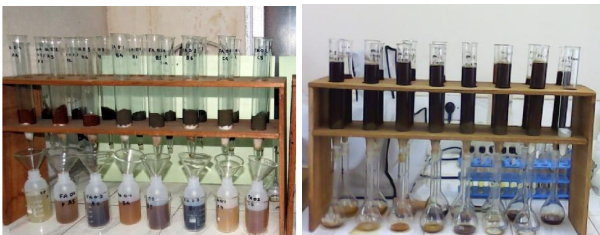
Fig. 3.8. Soil washing through column leaching technique with different extractants.
