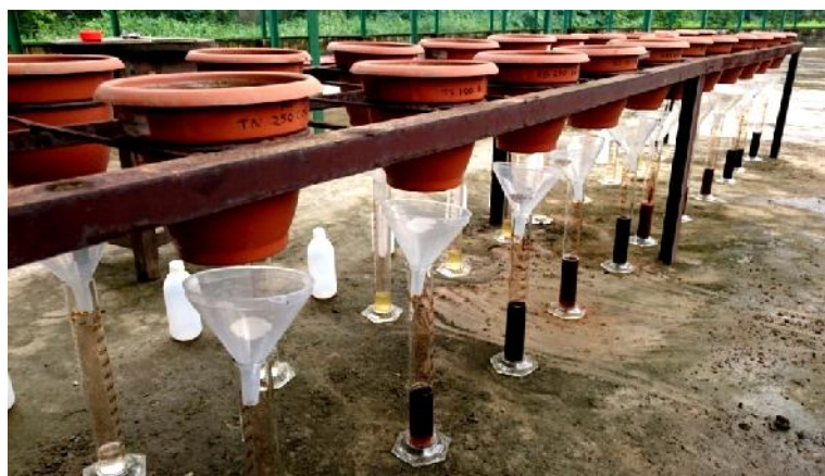
Fig 3.10. Collection of leachate after extraction with humic acid and combined extractants.
