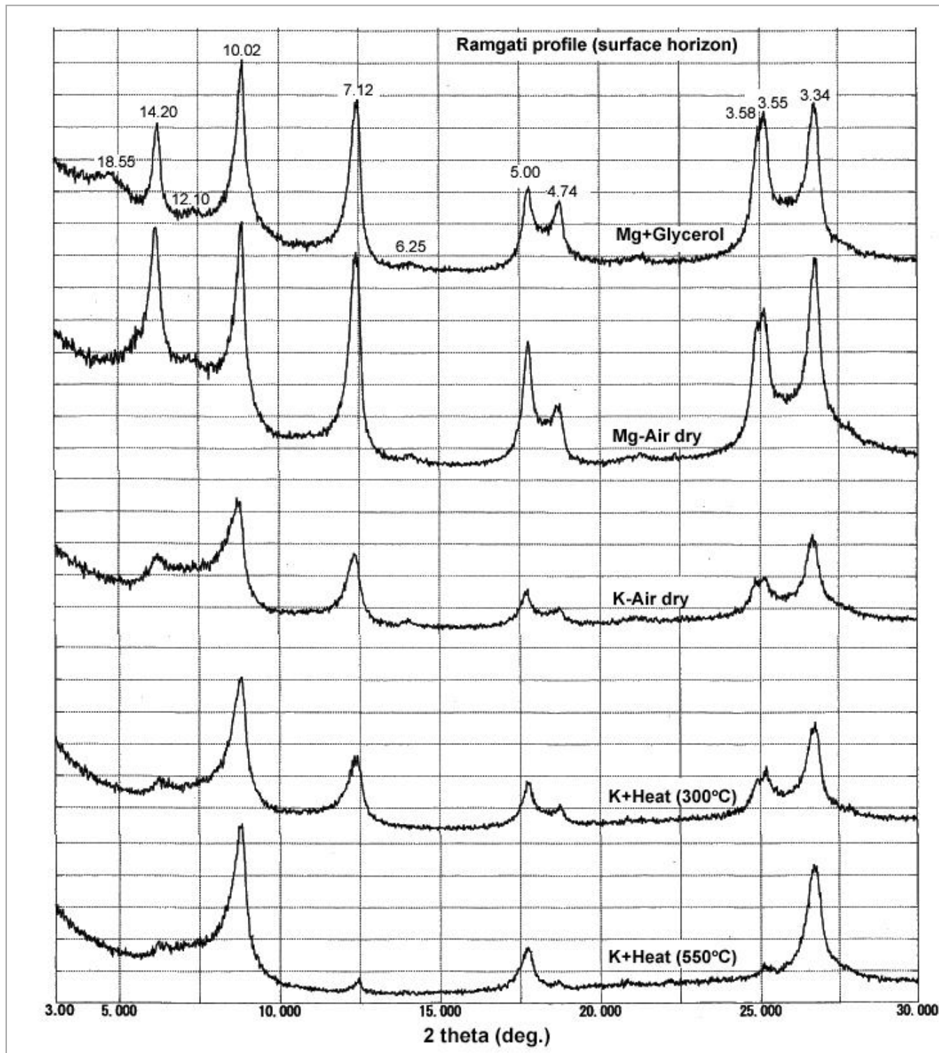
Fig 85. X-ray diffractogram of clay samples from Ap horizon of Ramgati series
