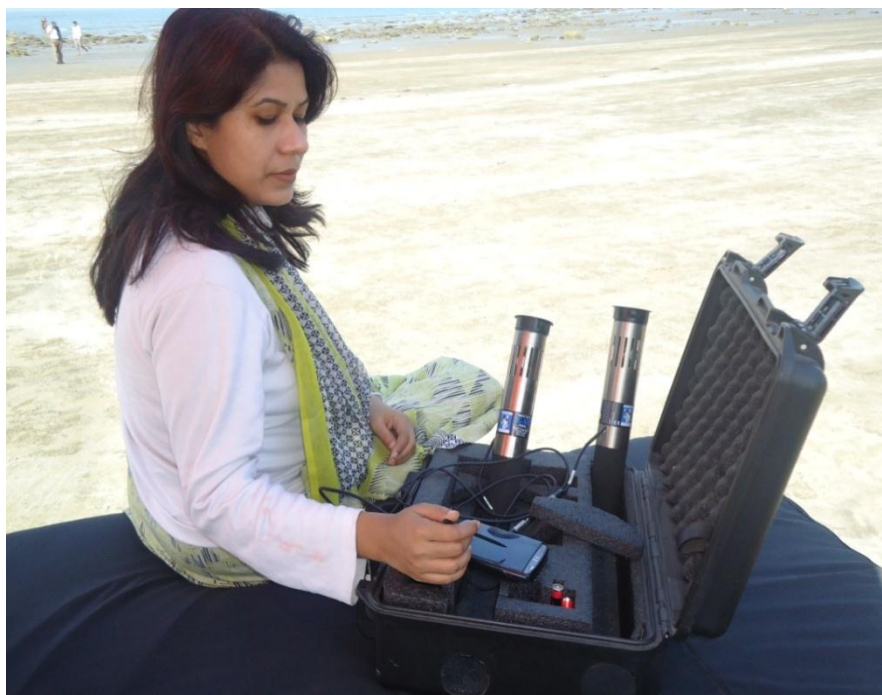
Fig. 3.3: Toxic gas (TG- 501 and TG-502 probes) monitoring equipment.
