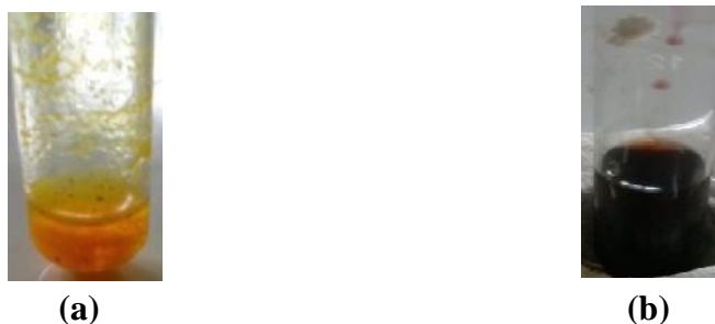
Figure 4.7. Chemical analysis: (a) orange precipitate formed on addition of 2,4-DNPH (b) solution turns from colorless to violet on addition of FeCl_3(aq) .
