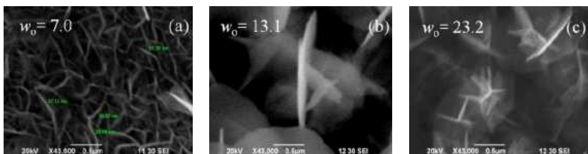
Figure 7.3.31. SEM images of the electrodeposited Co from 20 mM \text{Co}^{2+} in reverse microemulsions of CTAB with (a) w_o = 7.0 , (b) w_o = 13.1 and (c) w_o = 23.2 at -0.90 V (below the reduction potential) [93].
