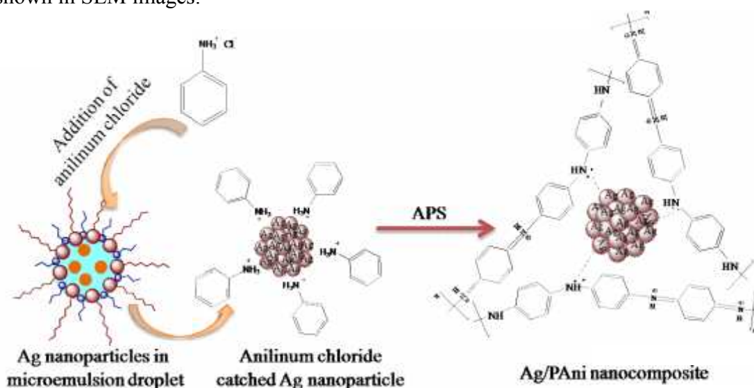
Figure 5.8. Mechanism of formation of Ag/PANI nanocomposite.
