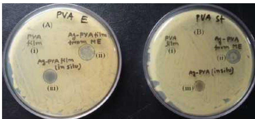
Figure 6.9. Antibacterial activity test against pathogens; (A) E. coli (B) S. aureus . Samples are labeled as: (i) PVA film as control (ii) Ag/PVA film from w/o microemulsion and (iii) Ag/PVA film from aqueous synthesis.
