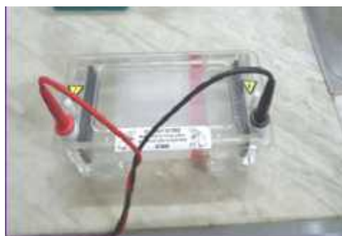
Fig.2.2. A Photograph of gel electrophoresis of PCR product at 120V for 60min
