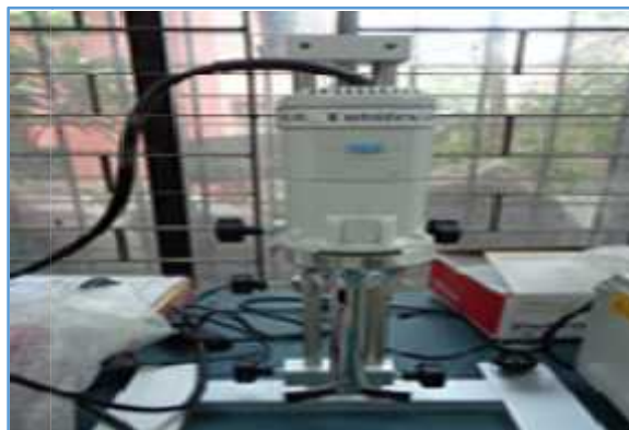
Figure 2.1 A photograph of electric homogenizer used for DNA extraction
