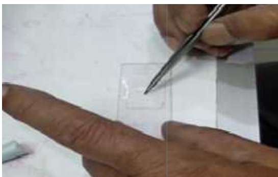
O. Mounting (cover slip) with Canada balsam
