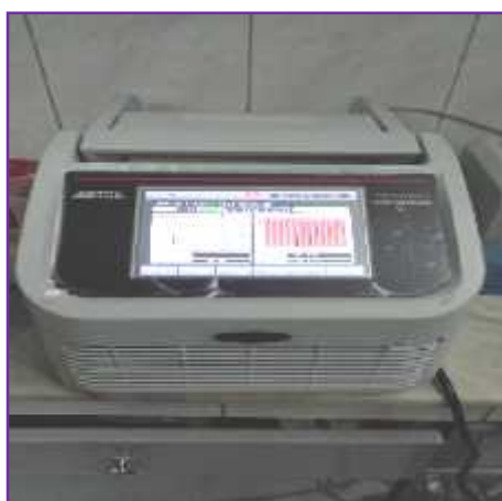
Fig. 2.1.A photograph PCR machine used for DNA amplification
