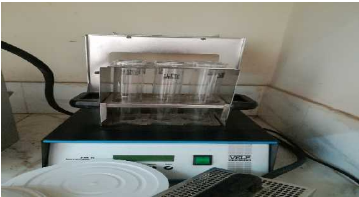
A: Digestion chamber
