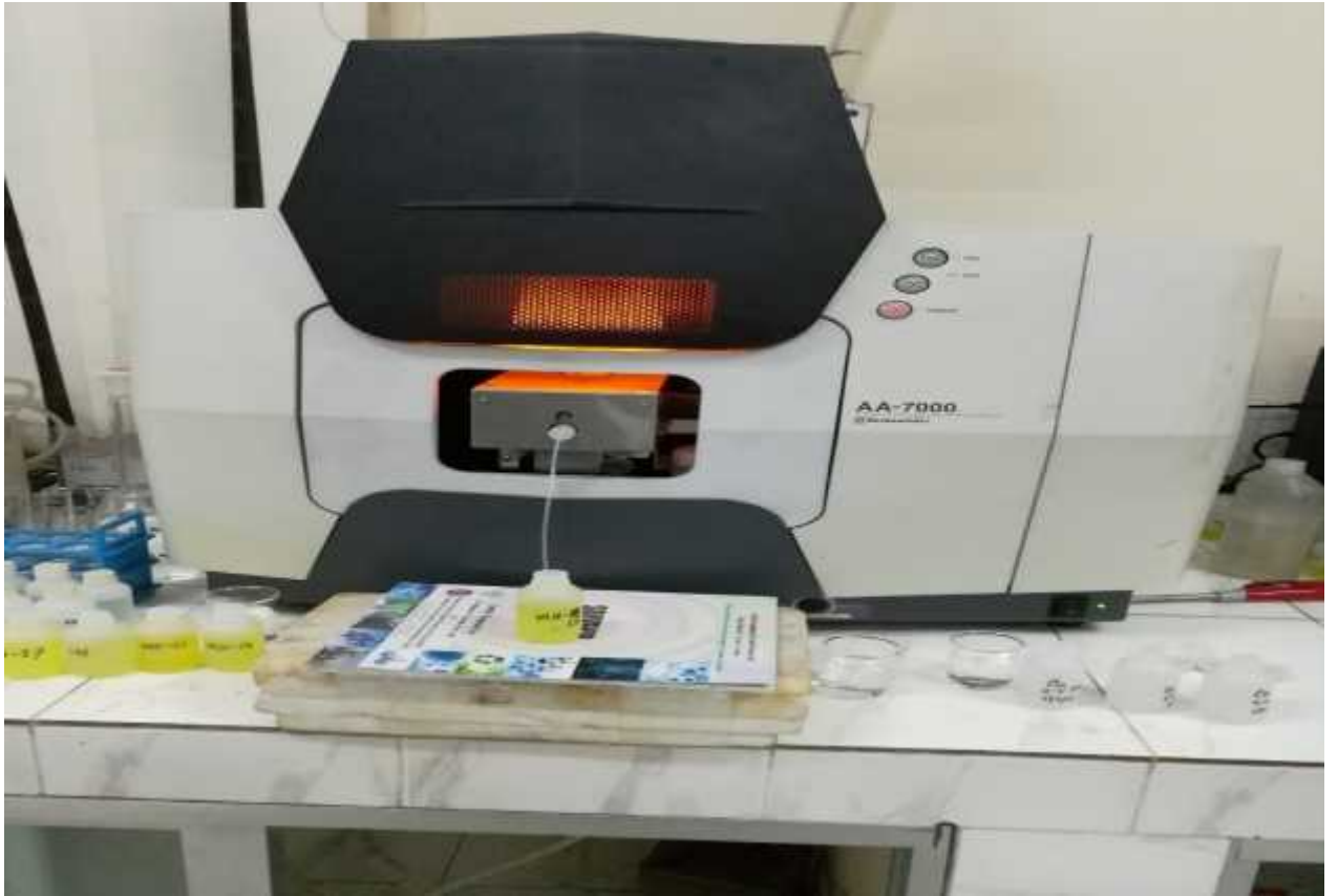
Plate 5: Atomic Absorption Spectrometer for minerals analysis
