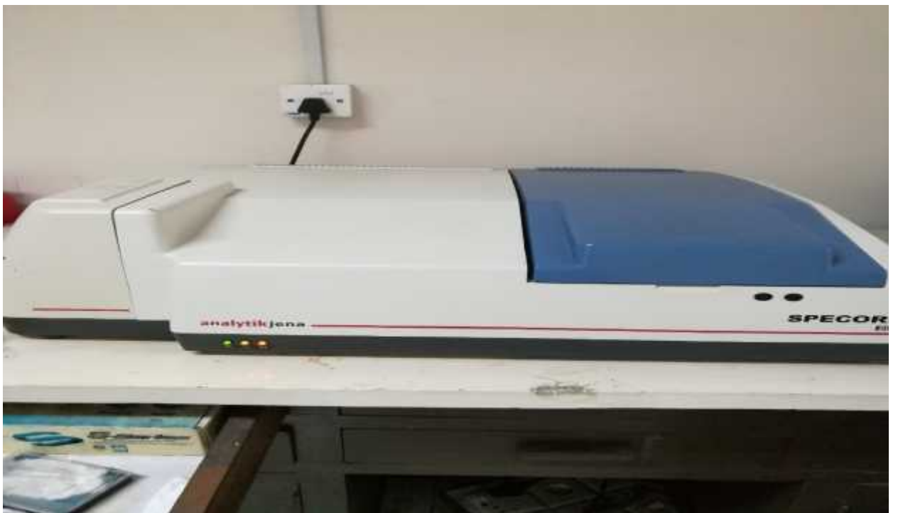
Plate 5: Atomic Absorption Spectrometer for minerals analysis
