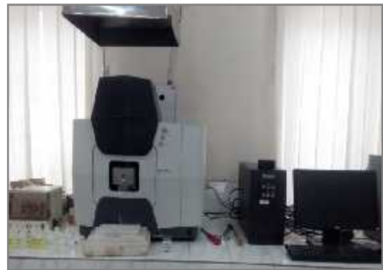
D. Determination of heavy metals in Atomic Absorption Spectrophotometer
