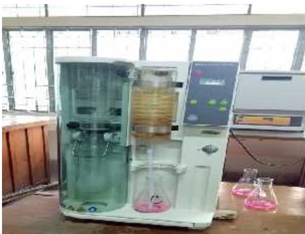
5E Unreacted H_2SO_4 titrated against NaOH
