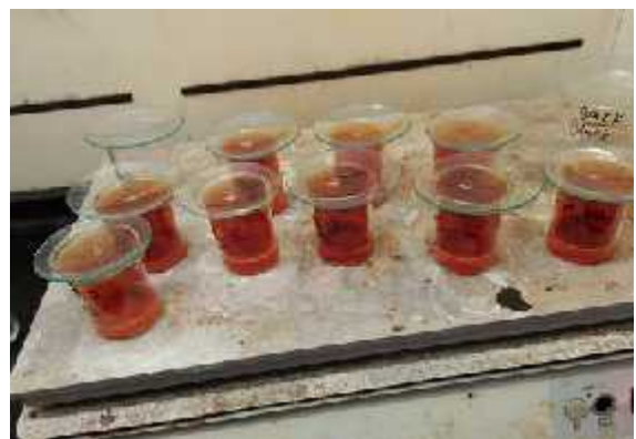
F. Digestion of samples in Fume chamber
