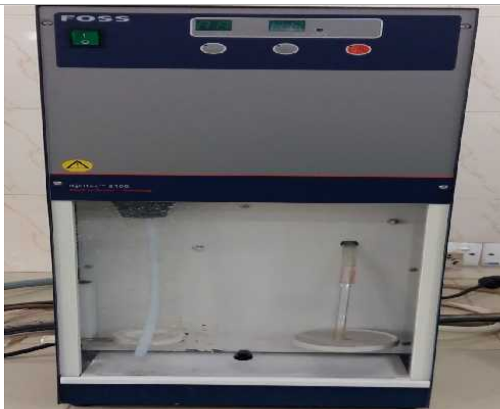
A. Digestion chamber
