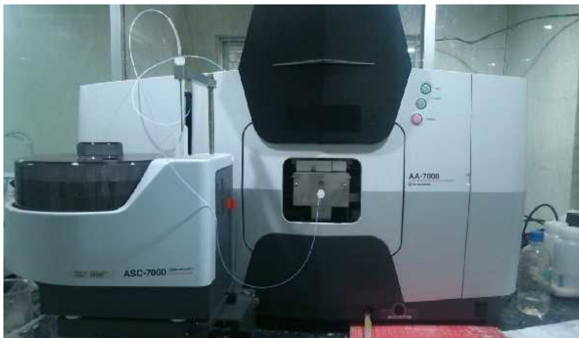
Figure 8: AAS used for metal analysis (Shimadzu AA-7000 )
