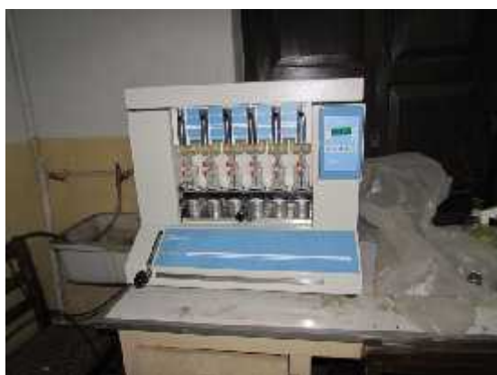
Lipid extraction by Soxhlet Method
