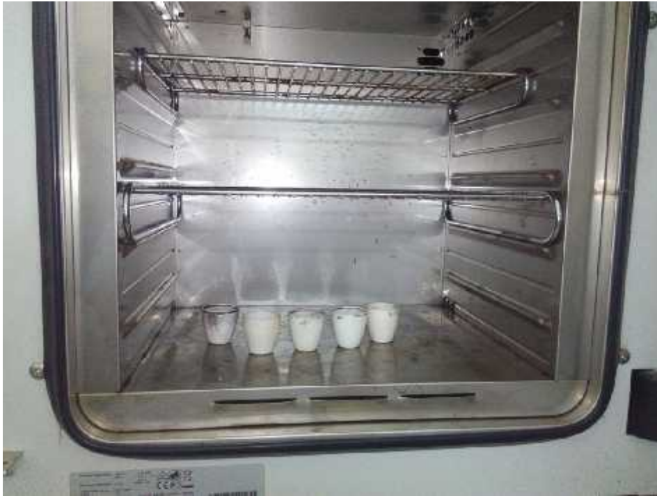
Plate 10: Crucibles are placed in the oven to determine the moisture content.
