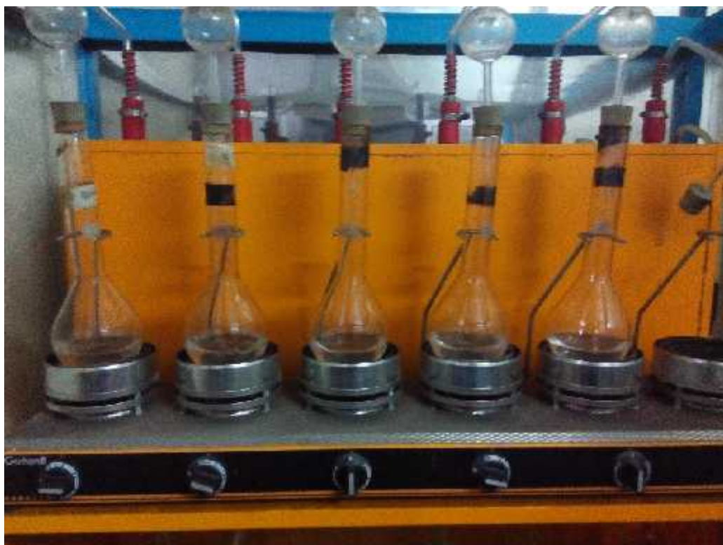
Plate 12: Kjeldhal flask distillation during the determination of protein content.
