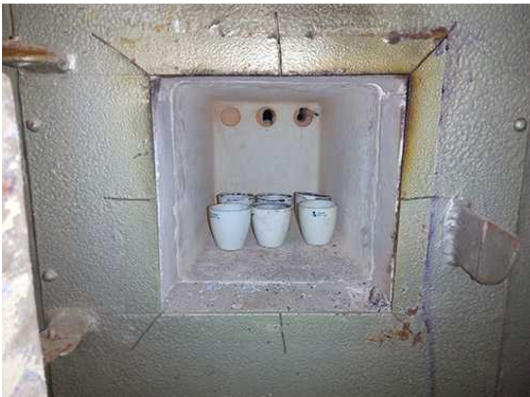
Plate 11: Crucibles are placed in the muffle furnace to determine the ash content
