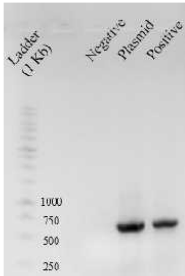
Figure 3.6 Representative gel autoradiograph showing amplicon of VP28 primer pair in gel purified plasmid. Amplicon size was about 643bp and 1 kbmarker used (Promega, USA).
