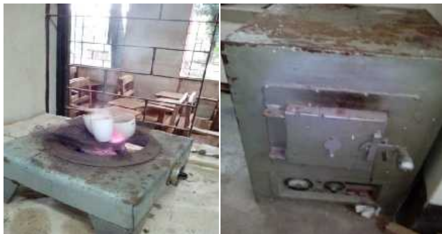
Burning of fish muscles for ash Muffle furnace
