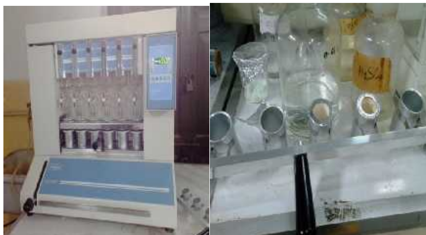
Soxhlet machine for lipid contents Fish muscles for lipid contents
