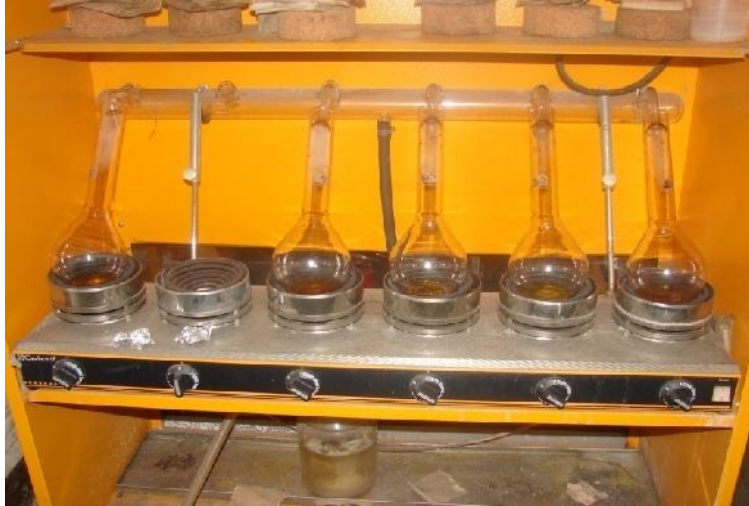
Figure: 2.3: Microkjeldhal digestion unit for the determination of protein content of fish
