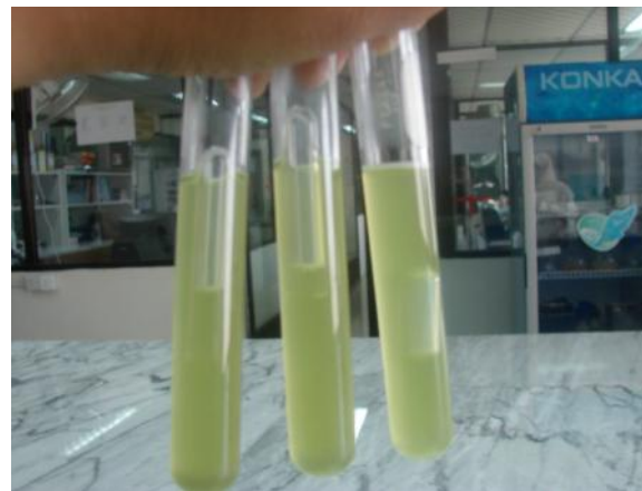
Plate 21. Gas Formation in BGGB after Incubation
